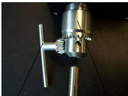
chuck key (B) Stirring tool (G) chuck (F)
